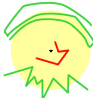
Figure 2 Drive test routes that are preferred (green) and not preferred (red) for measurement of a station’s HD Radio signal coverage area (yellow).
