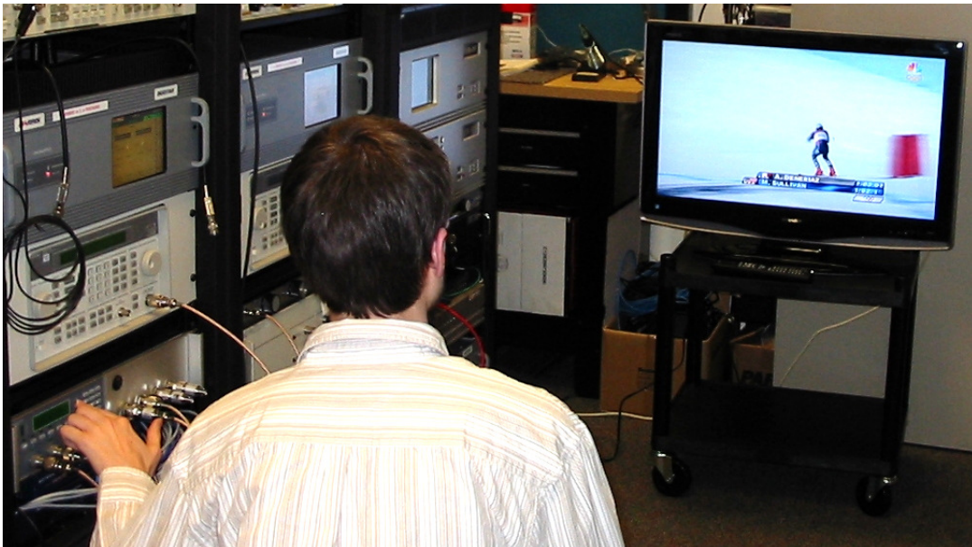
Figure 1 - Digital TV under test, viewed by test engineer
